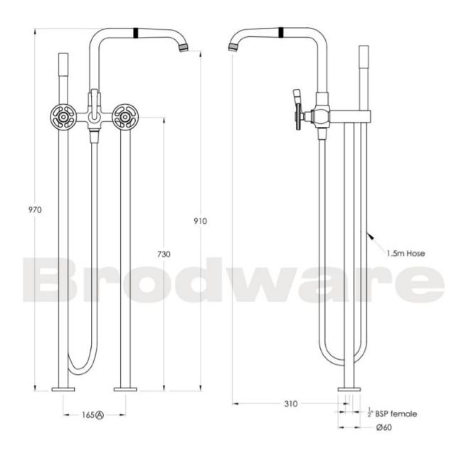
Note: G ½" BSP male thread required in the floor A Fixed Centre; taps must have 165 mm centres
